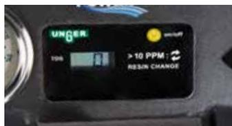
The **TDS meter** shows the water quality at water outlet for the Pure and the Boost Mode.
