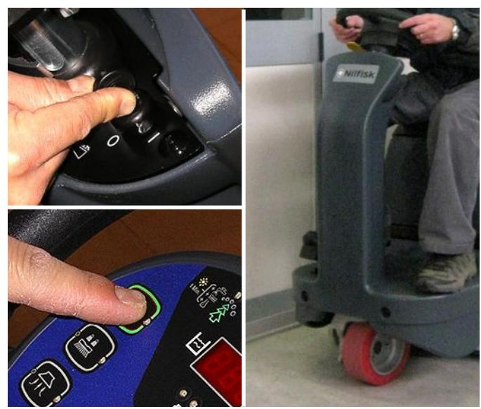
6. Turn the ignition key to "I", then lower the deck by pressing the Green switch. To engage the brushes, slightly press the pedal speed and then release it.
