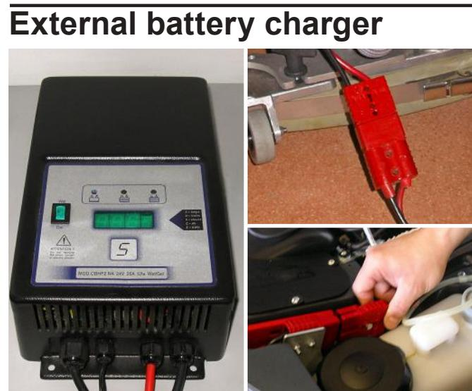
1a. Switch off charger by pressing the STOP button. Unplug charger cable from red battery plug. Reconnect the red battery plug to the machine.
