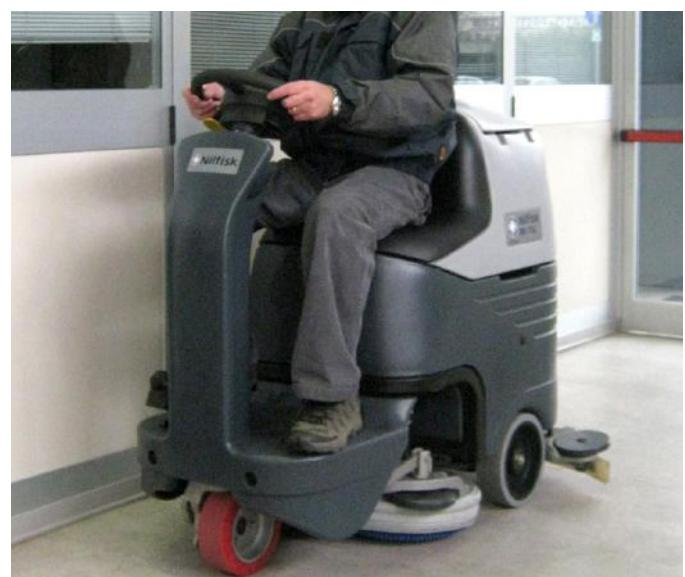
11. Push the pedal speed for starting floor cleaning. If solution applied flows outside the brush housing during use, reduce the flow of solution. Switch off the machine using the key.
