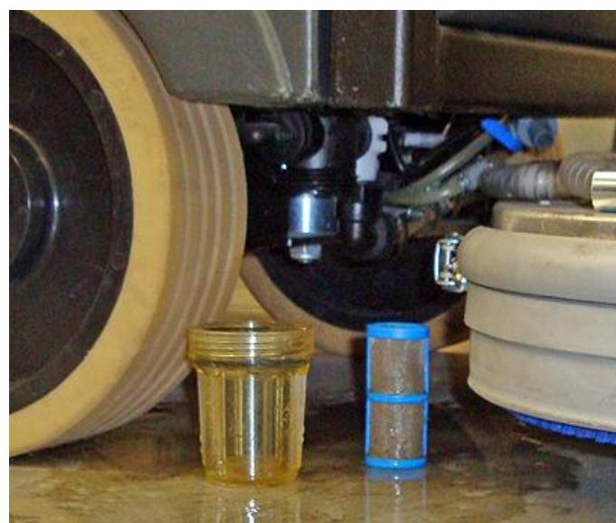
14. Clean the filter: 1) Close the solution tap under the machine. 2) Remove the transparent cover and the gasket, then remove the filter strainer.
