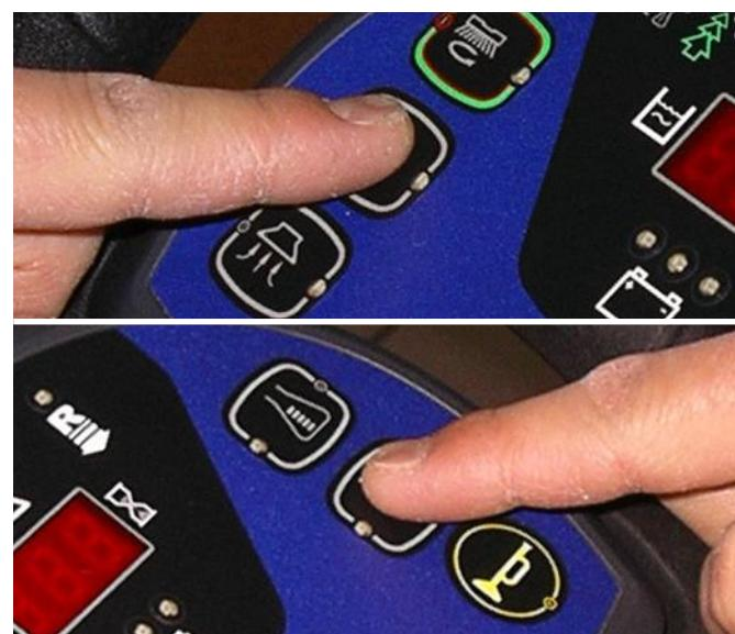
10. If necessary press the extra pressure function switch.
