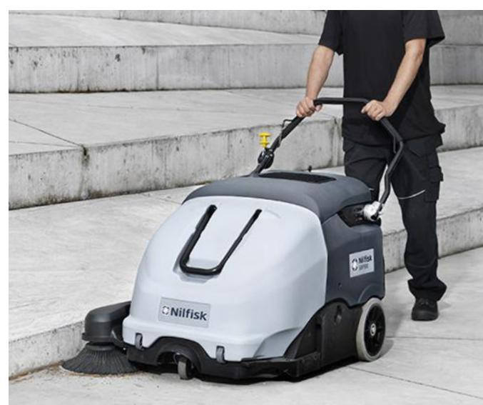
6. Drive the machine straight forward. Adjusting speed depending working conditions/quantity of debris.
