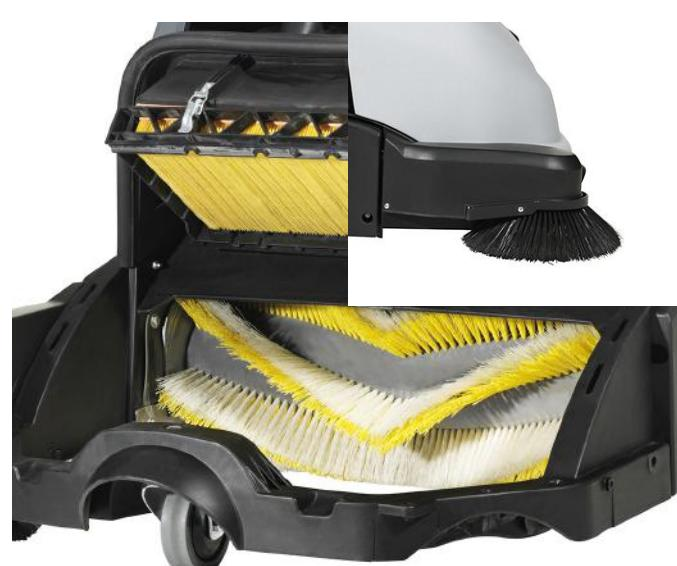
11. Check the main and side broom and remove any debris like straps, rope etc..
