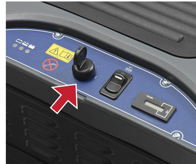
3. Turn the ignition key to "I" without pulling the drive control lever.
