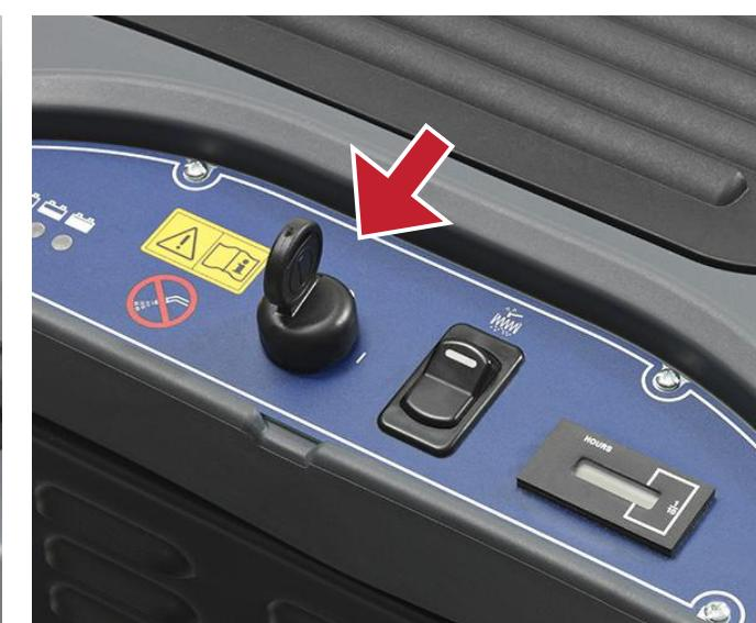
9. Release the traction lever, lift the side broom by and turn off the machine with the ignition key "0".
